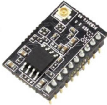
The WiFi module as shipped is pre-configured with Soft-AP enabled and the baud rate set to 9600. This should allow anyone with a WiFi enabled computer or laptop and a web browser to configure the WiFi module for your network. The procedure to use for that is shown below.
